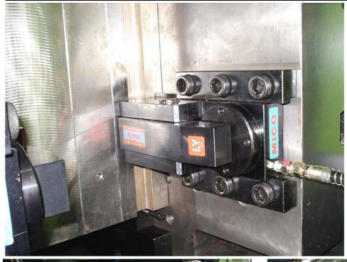
HYRobotics MICO-LYS Quick Mold Clamp is for molding machines without T-Slot on Mold platen. Durable Guide block allow the clamp moving forward/backward for quick mold change application for different size of mold in very short time.
