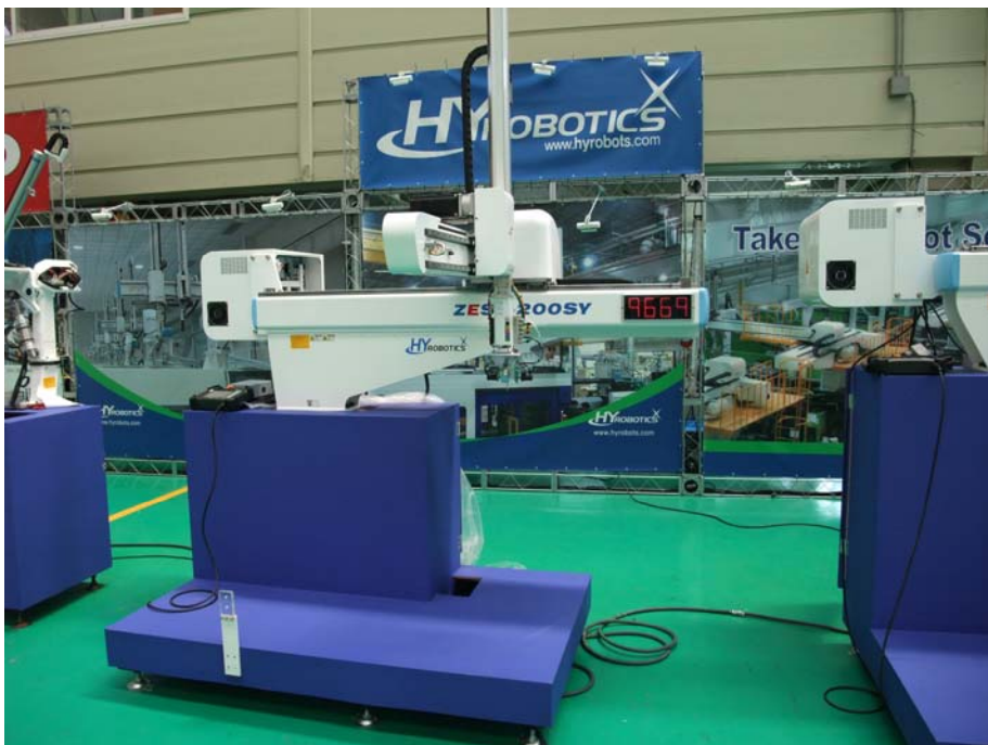
ZEST-200S : High Speed Take Out Robot for 100 ~ 250 Tons Machines
